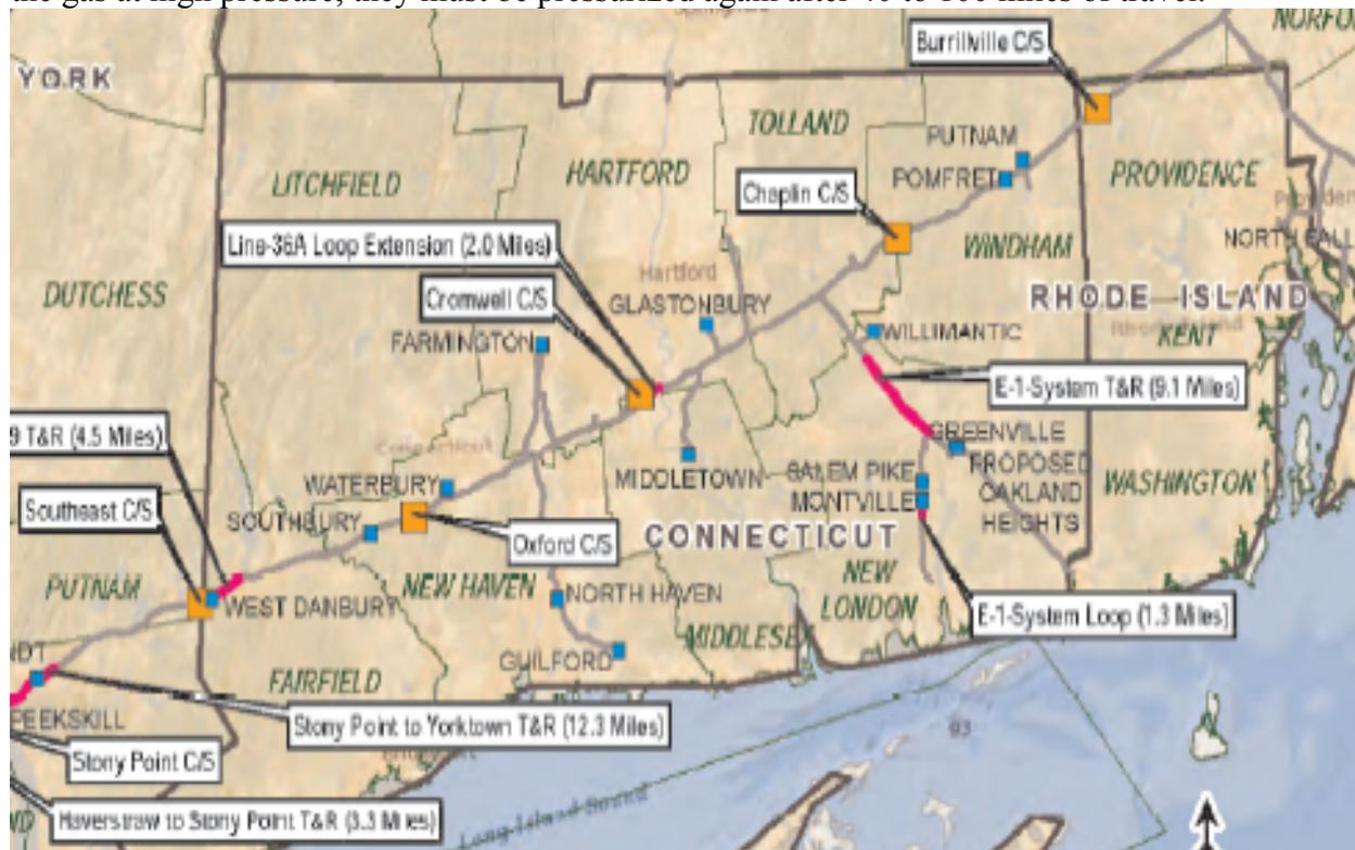
Branch transmission lines come off the main pipelines and carry gas to metering and regulations stations. The blue squares on the map above represent metering and regulations stations. At these stations, the high pressure of the gas is reduced to about 20 psi for distribution by local gas companies.
